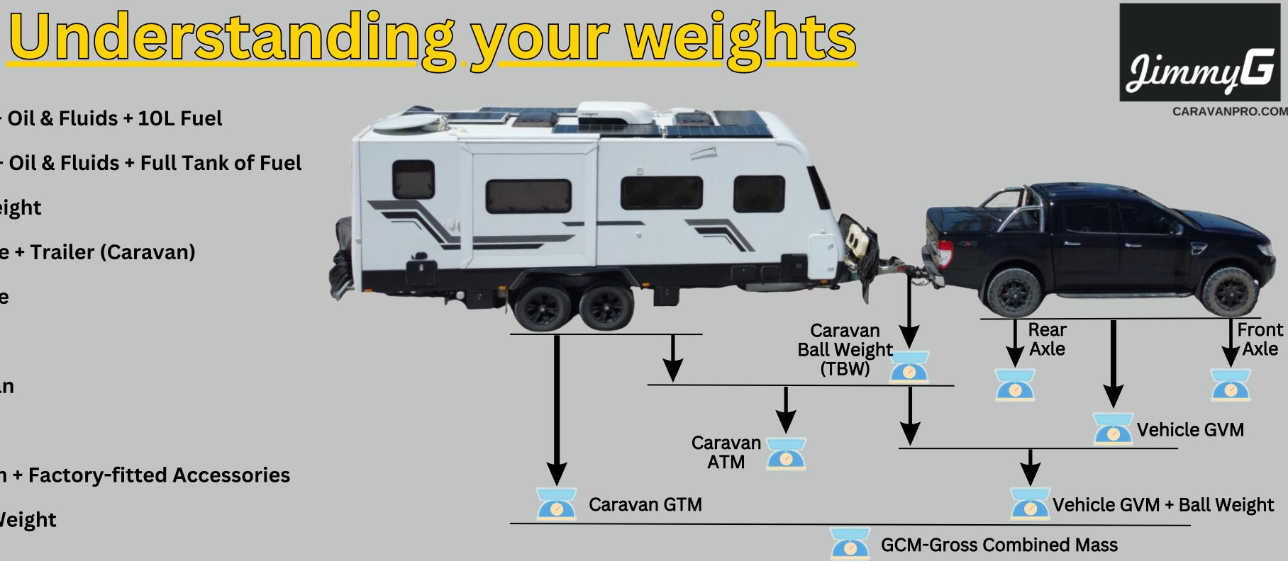
VEHICLE TARE WEIGHT = Weight of Vehicle + Oil & Fluids + 10L Fuel
